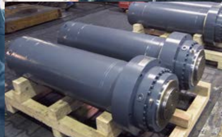
Cylinders for press in industrial laundry plant
